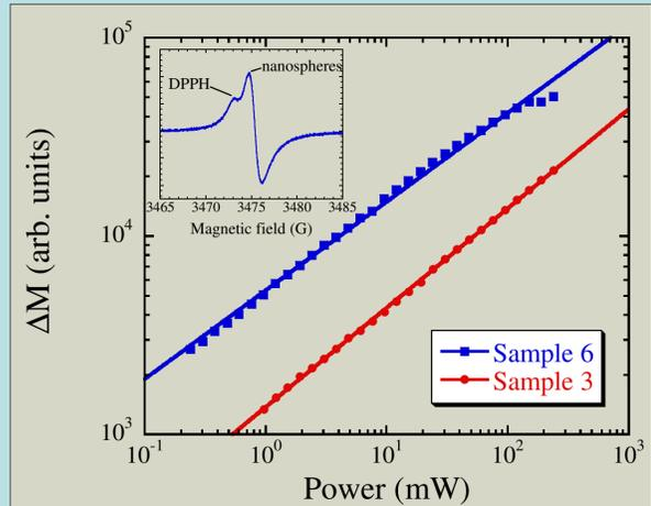
**Figure 4** CW-EMR power saturation curves for ammonia (Sample 3) and pyridine (Sample 6) nitrogen-doped CNS. There is a hint of saturation at the highest power values for Sample 6, but the data is not reliable enough to estimate relaxation times. The inset shows the EMR derivative curve for a composite sample of DPPH and Sample 6, showing that there is a small  $g$ -shift in this sample ( $-0.05 \pm 0.01$  %).
