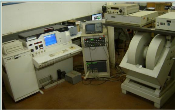
**Figure 1** Bruker ESP 300 E X-band spectrometer used to characterize the carbon nanospheres in this investigation.
