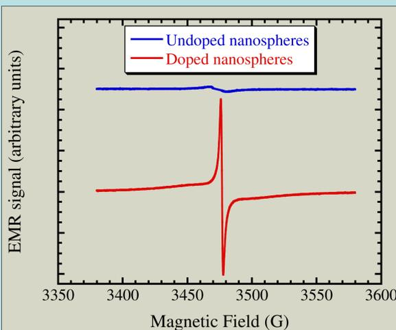
**Figure 2** EMR derivative curves for undoped and nitrogen doped CNS. The spectra were obtained using comparable spectrometer settings, and using a similar quantity of sample. The appearance of the strong paramagnetic peak supports our conclusion that the nitrogen occupies substitutional sites in the carbon matrix.
