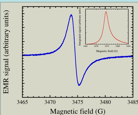
**Figure 3** EMR derivative curve for CNS doped with pyridine as the nitrogen source. The inset shows the integral of the experimental curve, and highlights the asymmetric (Dysonian) nature of the signal. Pyridine provides the most effective source of nitrogen for the CNS – the signal here is at least two orders of magnitude bigger than the signal obtained for the sample prepared using ammonia.
